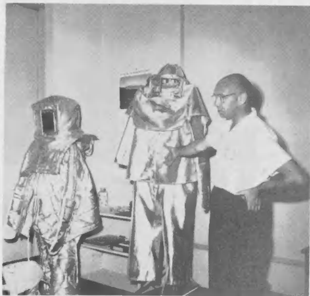
SPACE-SUITS? No, just a fire entry and proximity suit used by Lago fire fighters. Use of the latter suit is shown at right.
